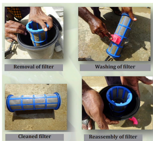
Figure 70: Sand Filter Cleaning Process (Source: Rashtriya Krishi Vikas Yojana) 110
